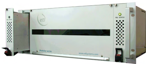
Front view of chassis with hot-swap PSU's
