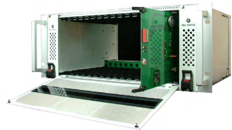
Front view showing hot-swap RF modules
