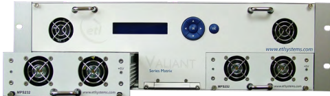
Front view showing hot-swap power supplies
