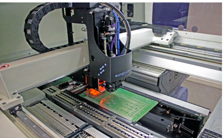
ETL's twin head pick and place machine capable of placing 32,000 components per hour
